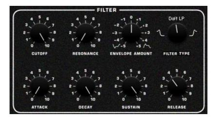
This section controls ATTACK, DECAY, SUSTAIN LEVEL and RELEASE of the Cutoff FREQUENCY, just like on the original Prophet 600. The ENVELOPE AMOUNT knob control the amount of EG (Envelope Generator) that modulates the Filter Cutoff FREQUENCY (how much "envelope" is "sent" to the Filter)
