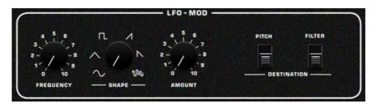
Similar to the original **Prophet 600**, there's a LFO which controls the **CUTOFF** of the Filter. LFO can be turned On and Off using the **LFO ON/OFF** button.
