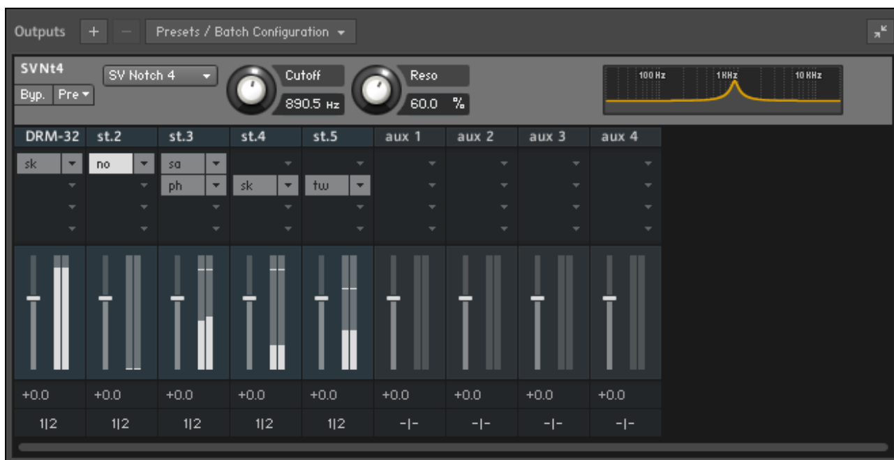
Example of Kontakt (standalone) with outputs assigned to multi-outs and additional effects on each output.
