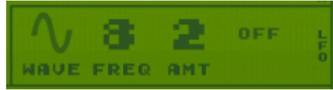
The LFO which controls the **CUTOFF** of the Filter. LFO can be turned On and Off using the small **ON/OFF** button.
