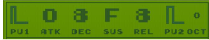
This section contains **Waveform selectors** for Pu1 and PU2.
